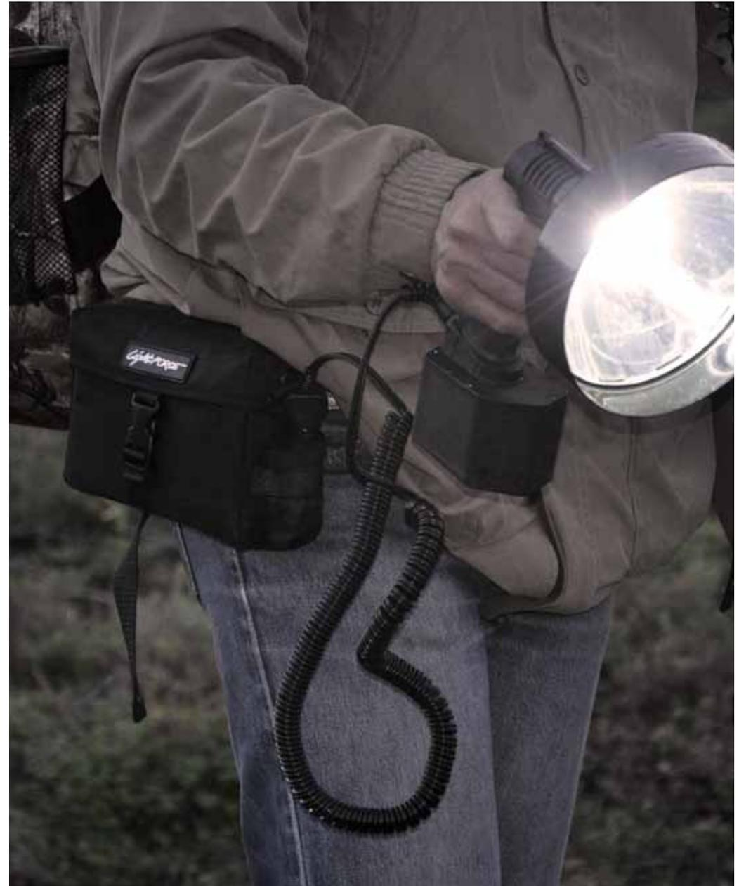
Built within this battery is an onboard battery management system that monitors the individual cells and then calculates total remaining capacity via the onboard LED display. You'll never be caught short with the Lightforce In Field Power Pack.
