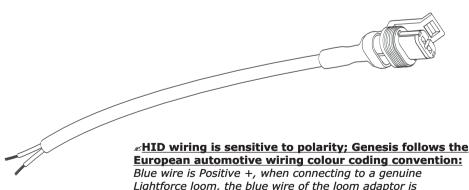
Lightforce loom, the blue wire of the loom adaptor is connected to the white wire of the loom. The brown wire is negative -, this must be connected to the black cable of the vehicles loom.
